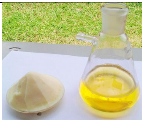
Figure 13: Shea Stearin (left) and Olein (right) fractions from the optimized process
