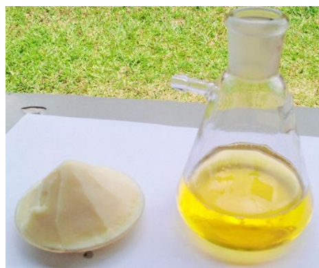
Figure 5: Shea Strain (left) and Olein (right) fractions from the optimized process
