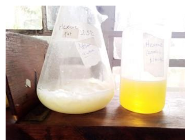
Fig 14: Fractionated shea butter into olein and stearin with hexane
