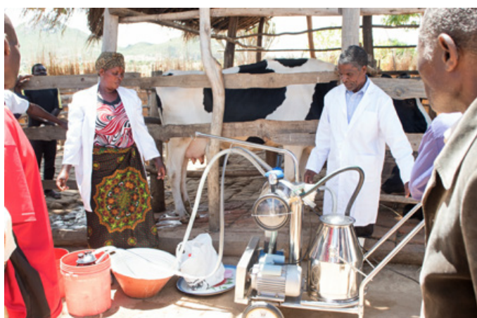
Figure 2: Solar powered milking machine
